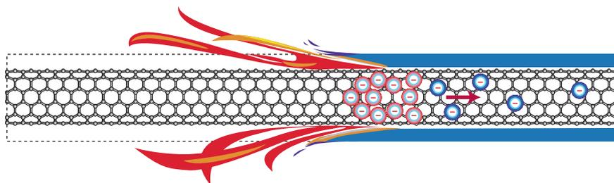
**Figure 1** | A chemically driven thermal wave (shown in red) generates thermally excited electrons in a thermopower wave; its propagation to the cold (blue) end of the nanotube can be harvested as electrical energy. Figure courtesy of Ali E. Aliev.
