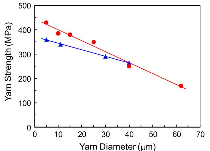
**Figure 3.** Dependence of yarn tensile strength on yarn diameter for low twist yarns (circles, for helix angle  $\alpha \sim 15^\circ$ ) and high twist yarns (triangles, for helix angle  $\alpha \sim 50^\circ$ ). The forest used for spinning had a height of 350 μm, which is the nominal nanotube length.
