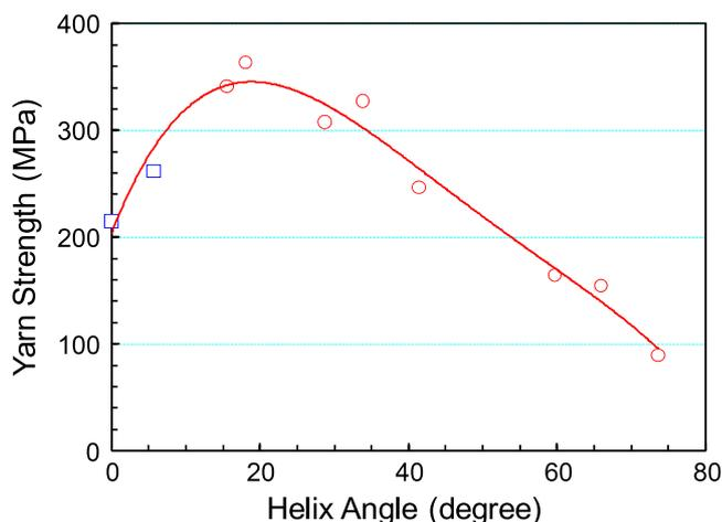
**Figure 4.** Dependence of yarn tensile strength on yarn helix angle for forest-spun MWNT yarn. Yarns having very low twist (squares) were liquid densified before twist insertion, and the remaining yarns (circles) were twist-spun without any prior treatment. The yarn diameter was kept constant at  $\sim 20 \mu\text{m}$ . The forest used for spinning had a height of  $350 \mu\text{m}$ , which is the nominal nanotube length.
