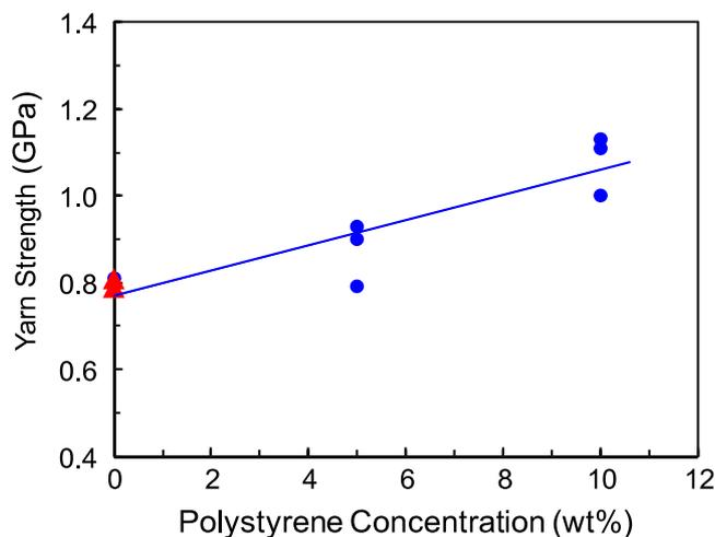
**Figure 5.** Tensile strength of  $\sim 4.5 \mu\text{m}$  diameter polystyrene-infiltrated MWNT yarns as a function of the concentration of the polystyrene solution. Closed circles show yarns infiltrated with polystyrene/chloroform solution. Triangles correspond to yarns that have not been solution-treated.
