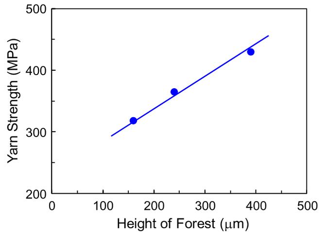
**Figure 2.** Dependence of the strength of a twist-spun MWNT yarn on forest height for MWNT forests grown by CVD of acetylene gas. All tensile strengths are for yarns with about the same helix angle (17°–21°) and diameter (5–7 μm).
