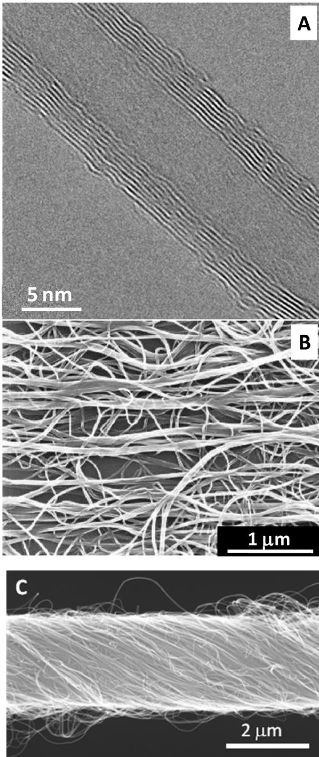
**Figure 1.** (A) Transmission electron microscope image showing an MWNT from a forest used to produce yarn, (B) an SEM image of a forest-drawn MWNT aerogel sheet strip that can be densified to make a yarn and (C) an SEM image of an MWNT yarn that was twist spun from such an MWNT aerogel sheet strip.
