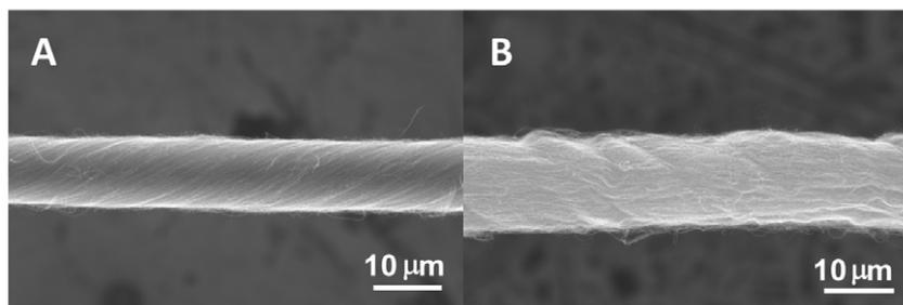
**Figure 6.** SEM images of (A) true-twisted yarn with  $26\,000 \text{ turns m}^{-1}$  twist and (B) false-twisted yarn obtained by insertion of  $26\,000 \text{ turns m}^{-1}$  twist, followed by removal of this twist by twist insertion in the opposite direction.
